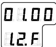
4. Confirm the entry by pressing the **ACK/ENT** button. The display will return to sub-category **1.1.U**, and the data will be transferred to the gyro immediately.
